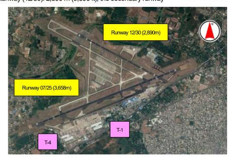
The airport has 24 taxiways, capable of handling 36 aircraft movements per hour on primary runway and 25 aircraft movements per hour on secondary runway. In January 2018, the airport began cross-runway operations to avoid flight delays, increasing aircraft movements from 36 to 42 an hour.
